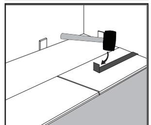
**Step 9:** Use hammer and pull bar to lock long edges of planks on final row.
