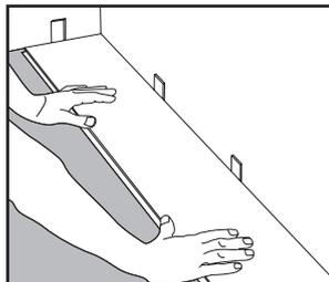
**Step 2:** Lock short end of plank by tapping down the ends until they lock into place. Continue to end of first row.
