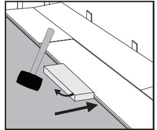
**Step 6:** Attach a scrap piece of floor to bridge gap between ends of planks.
