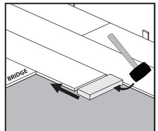
**Step 8:** Use hammer and pull bar to lock final piece in row. Insert spacer at end of row. Continue installation to final row.
