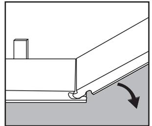
**Step 3:** Use leftover plank from first row as starter for second row. There must be at least 300mm between plank end joints on adjacent rows.
