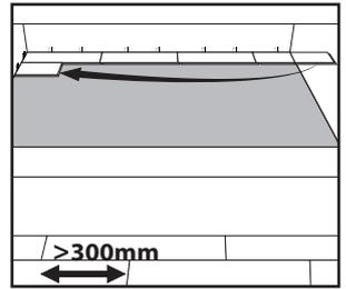
**Step 4:** Lock long edge of plank by inserting tongue into groove and drop in place.
