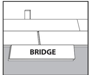
**Step 7:** Tap end of plank with hammer and tapping block to lock ends of planks together. Remove bridge and continue towards wall until installing the final plank in the row. BE SURE TO TAP ON EDGE OF VINYL SO AS NOT TO DAMAGE LOCKING PROFILE.
