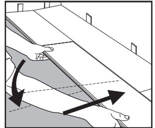
**Step 5: IMPORTANT!** Use hammer and tapping block to tap long edge of plank to ensure a tight fit. ANY GAPPING CAN COMPROMISE THE LOCKING SYSTEM!
