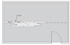
Score a line on the last plank, then deep cut along the line. Continue this way until you have at least three rows complete. Mark a pencil line along the last row and remove the planks keeping them in the correct order for placement.
