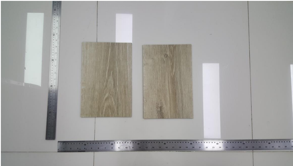
Photo 1. Tested sample – SPC VINYL FLOORING (item no.: KC1522)
