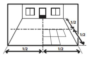
Carefully measure the width of the room and mark the centre line, determine the width of the last row of the tiles. If the width of the last row is less that 50mm, the width of the first row should be adjusted to allow a larger cut.
